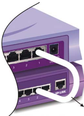
Fig. 4-1 Uplink to another Switch/Hub using straight-through cable
